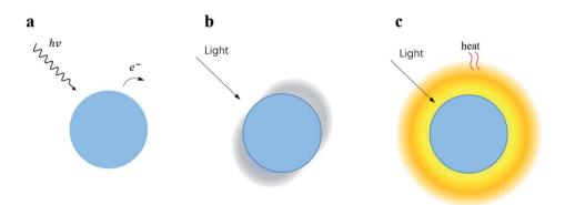
Fig. 4 Triple excellent characteristics of LSPR. Mechanism A: a photo-induced hot electron can be transferred from the NP under visible light. Mechanism B: the enhancement of the local electromagnetic field at the vicinity of the NP helps reduce the electron-hole recombination. Mechanism C: the photo-induced temperature increase of the NP provides heat to the reaction system. Reprinted from ref. 44. Copyright 2014, Chemical Society.
