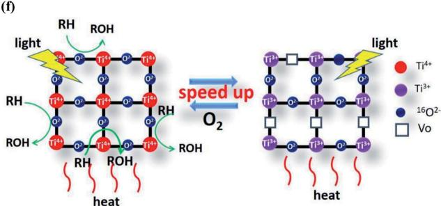
Fig. 10 (a) Experimental diagram of photo(thermal)catalytic degradation of  $CH_3CHO$ . (b)–(e) Photo(thermal)catalytic degradation rate of  $CH_3CHO$ . (f) Mechanism diagram of surface lattice oxygen of  $TiO_2$  participating in the photothermal catalytic oxidation reaction. Reprinted from ref. 123.
