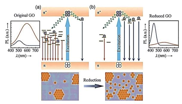
Fig. 5 Proposed PL emission mechanisms of (a) the predominant "red emission" in GO from disorder-induced localized states and (b) the predominant "blue emission" in reduced GO from confined cluster states.<sup>221</sup> Adapted from ref. 221 with permission from John Wiley and Sons, copyright 2021.
