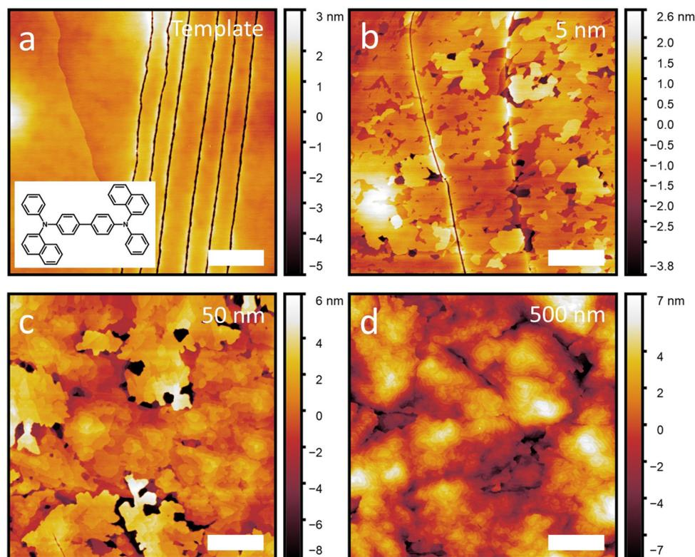
Fig. 1 Atomic force microscope images of an (a) NPB template crystal and (b) 5 nm, (c) 50 nm and (d) 500 nm of additional NPB grown on top of the template. Scale bars are 1  $\mu$ m. Molecular structure of NPB is shown as an inset in (a).
