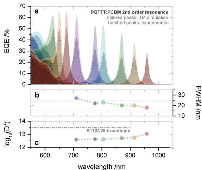
**Fig. 11** Solution processed PBTTT:PC<sub>61</sub>BM CT-OPDs based on the second order resonance. (a) Simulated and experimental (hatched) resonance wavelength and correlated EQE curves. The wavelength tunability in range of 650–910 nm was realized by varying the active layer thickness from 290–440 nm. (b) Corresponding FWHM and (c)  $D^*$ . Reproduced with permission.<sup>74</sup> Copyright 2017, WILEY-VCH GmbH.
