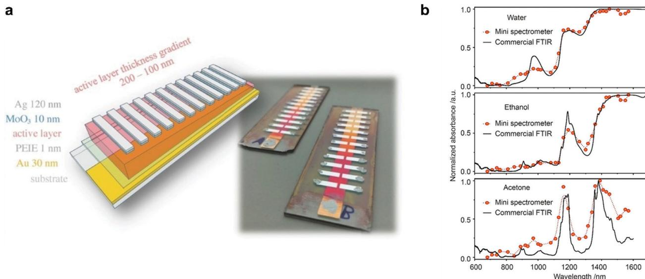
**Fig. 19** (a) A schematic and a photograph of a miniaturized spectrometer based on cavity enhanced NIR OPDs.<sup>74</sup> (b) Absorption spectra of water, ethanol, and acetone measured using the miniaturized spectrometer compared to the spectra measured with a commercial Fourier transform infrared spectrometer.<sup>18</sup> (a) Reproduced with permission.<sup>74</sup> Copyright 2017, WILEY-VCH GmbH. (b) Reproduced with permission.<sup>18</sup> Copyright 2021, American Chemical Society.
