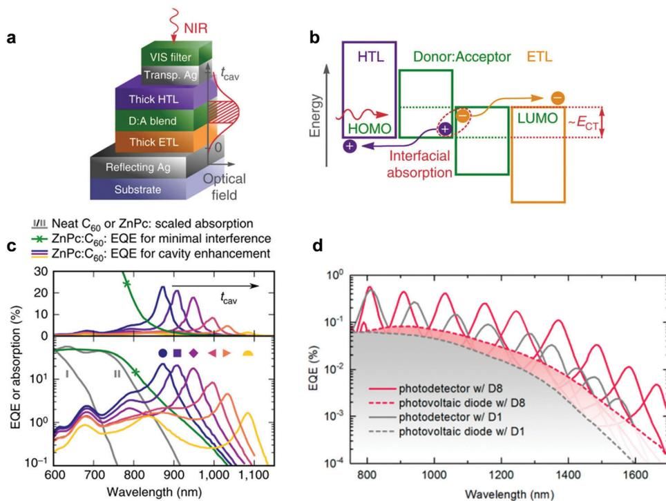
Fig. 10 (a) Simplified device architecture of a microcavity enhanced narrowband NIR OPD. (b) Schematic energy level diagram of the main materials involved in the OPDs. (c) NIR OPDs based on ZnPc:C<sub>60</sub> CT state absorption. (d) NIR OPDs based on the CT absorption of D8:C<sub>60</sub>. Subfigures (a–c) are reproduced with permission.<sup>27</sup> Copyright 2017, Springer Nature. Subfigure (d) is reproduced with permission.<sup>197</sup> Copyright 2019, American Chemical Society.
