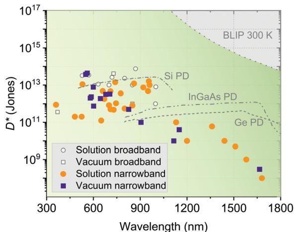
Fig. 15  $D^*$  as a function of wavelength based on different device processing methods (solution vs. vacuum processing) and photodetecting wavelength bandwidths (broadband vs. narrowband detection). Further details about the individual devices are given in Table 2. The  $D^*$  of Si, InGaAs and germanium (Ge) are extracted from ref. 138. The BLIP limit is calculated at 300 K for photovoltaic PDs with a field-of-view of  $2\pi$ .
