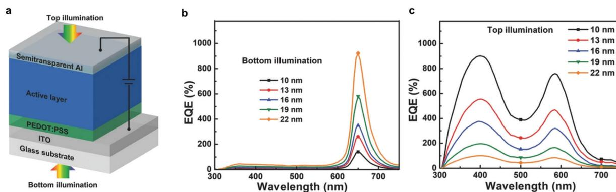
Fig. 7 (a) CIN-PM-OPD structure. EQE of the CIN-PM-OPD under (b) bottom and (c) top illumination. Reproduced with permission.<sup>193</sup> Copyright 2018, Wiley-VCH GmbH.
