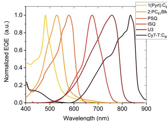
Fig. 5 Normalized EQE of OPDs based on narrow-photo-absorbing materials as a function of wavelength. 1(Pyrl):C<sub>60</sub><sup>177</sup> and Cy7-T:C<sub>60</sub><sup>22</sup> are PHJs. 2:PC<sub>61</sub>BM<sup>21</sup> is a BHJ blend. PSQ<sup>19</sup> and ISQ<sup>20</sup> are single-component photo-absorbing materials with D–A–D chemical structure and U3 is also single component device.<sup>23</sup>
