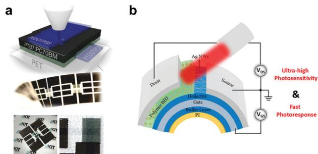
**Fig. 16** (a) Schematic structure and photographs of fully-printed ITO-free OPDs on PET foil showing their semi-transparency and mechanical flexibility.<sup>216</sup> (b) Device structure of flexible PT-OPDs with ultrashort channel length.<sup>217</sup> (a) Reproduced with permission.<sup>216</sup> Copyright 2015, WILEY-VCH GmbH. (b) Reproduced with permission.<sup>217</sup> Copyright 2018, American Chemical Society.
