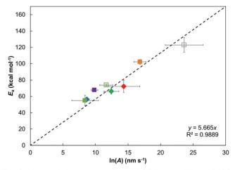
Fig. 6 Linear relation between  $E_a$  and ln(A) for the different ZDDPs studied, suggesting a kinetic compensation effect.<sup>82</sup> Vertical and horizontal bars show 95% confidence intervals. Legend is the same as in Fig. 5, closed symbols use  $\Delta V^*$  calculated at 80 °C, open symbols at 120 °C.
