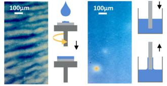
Spin-coating 2x deposition a 1.5 min Dip-coating 4x deposition a 7 min
