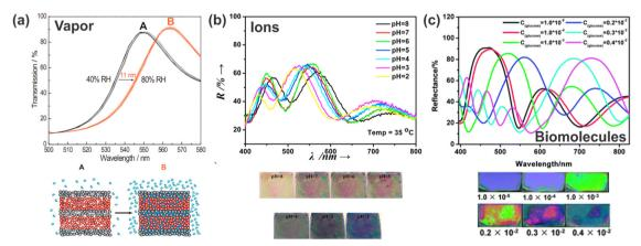
Fig. 9 Response of 1DPCs to different chemical stimuli: (a) relative humidity; adapted and reprinted with permission from ref. 102, Copyright 2011 American Chemical Society. (b) H<sup>+</sup> ions; adapted and reprinted with permission from ref. 103, Copyright 2015 Elsevier. (c) Glucose oxidase (GO<sub>x</sub>); adapted and reprinted with permission from ref. 104, Copyright 2012 Royal Society of Chemistry
