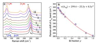
**Fig. 6** (a) Raman spectra of CANBIC perovskites with varied Bi fraction y=0 (1), 0.01 (2), 0.05 (3), 0.07 (4), 0.10 (5), 0.15 (6), 0.20 (7), 0.50 (8), 0.80 (9), and 1.00 (10). (b) Frequency of the  $A_{1g}$  mode as a function of Bi fraction y (scatter). Solid red line represents the best fit with a polynominal function " $\nu(A_{1g})$  versus y" presented in the figure.
