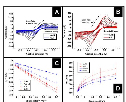
Fig. 4 (A) CV data for example NA-AMEs; (B) CV data for example A-AMEs; (C) Randles-Ševćik plot for the AMEs based on the average data from CV; (D) average  $\Delta E_{\rm p}$  versus scan rate for the AMEs. For (C and D), the data points are (Mean  $\pm$  S.D.).
