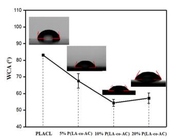
Fig. 3 Water contact angle of the blends.
