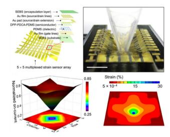
**Fig. 13** Architecture, photograph, normalized on-current, and simulation results of strain applied by poking with a plastic bar to the fully stretchable active-matrix TFT array containing self-healable semiconducting polymer. <sup>31</sup> Copyright: 2019, Science Advances.
