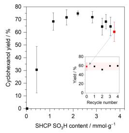
Fig. 4 Cyclohexanol yield of SHCP catalysed hydrolysis of cyclohexyl acetate as a function of  $\rm SO_3H$  content. The inset shows the catalytic performance of recycled SHCP-10 in the same conversion over four cycles.
