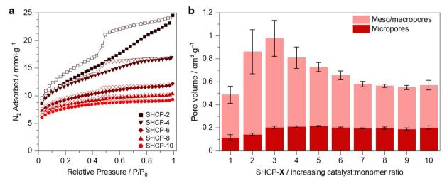
Fig. 2 Textural properties of SHCPs: (a) N<sub>2</sub> adsorption—desorption isotherms for a selection of SHCPs, the remainder are shown in Fig. S4 (ESI†). Filled symbols represent adsorption and empty symbols represent desorption. (b) Pore volume of all SHCPs divided into micropore contributions (red) and mesopore/macropore contributions (pink).
