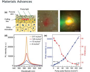
Fig. 18 (a) Schematic of random lasers implanted into the skin. (b) Optical microscope image of a laser embedded below the porcine skin surface. (c) PL image of the sample upon optical excitation. (d) Emission spectra of the embedded laser sample at various pump fluences. (e) Peak intensity and FWHM of emission spectra versus pump fluence. (Reproduced from ref. 74, with permission from [Elsevier]).
