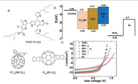
Fig. 1 (a) The molecular structures of D,  $A_1$ , and  $A_2$ ; (b) the device structure with the HOMO and LUMO energy levels ( $A_1$  and  $A_2$ ,  $A_2$ ) and work functions of various layers; and (c) illuminated J-V characteristics for different  $A_1:A_2$  ratios in D polymer based solar cells under AM1.5 illumination.
