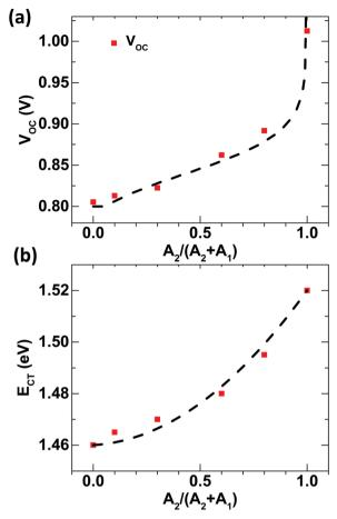
Fig. 2 Alloy composition vs. (a) changes in  $V_{\rm OC}$  using the double-diode model (the dotted line represents the fitting of experimental  $V_{\rm OC}$  values with eqn (2)) and (b) changes in the  $E_{\rm CT}$  value of the BHJ alloy composition determined from sensitive EQE studies (the dotted line represents the fitting of experimental  $E_{\rm CT}$  values with eqn (3).
