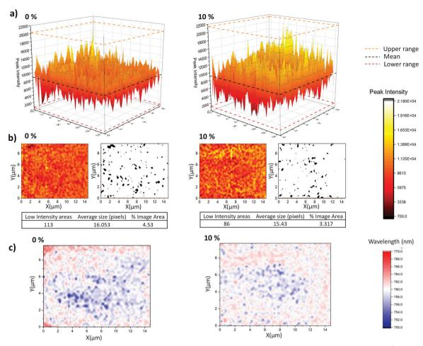
Fig. 7 (a) 3D plots of mapped PL intensity of MAPbl $_3$  crystallised from GVL only and GVL-10MeOH in ZrO $_2$  films across a 200  $\mu$ m $^2$  area, (b) 2D maps, with adjacent black and white images highlighting pixels in the bottom 10% of the PL intensity range. The corresponding tables detail the quantity, average size and overall coverage of these poorly infiltrated low intensity regions, (c) 2D contour maps showing the direction and intensity of peak shifting across the area.
