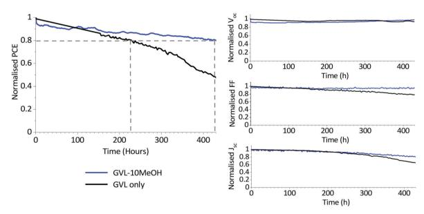
Fig. 9 Normalised PV parameters of an unencapsulated GVL only and GVL-10MeOH device over 430 hours of stability testing. Devices were tested every four hours and held at  $V_{oc}$  under AM1.5 illumination at 50 °C in ambient conditions for the duration. The dashed lines highlight device T80 lifetimes.
