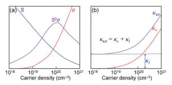
Fig. 1 (a) Illustrations of the trade-off relationship between the Seebeck coefficient (S) and electrical conductivity ( $\sigma$ ). (b) Variation in the thermal conductivities ( $\kappa_{c}$  and  $\kappa_{tot}$ ) as a function of the carrier density. Reproduced with permission from ref. 14, Copyright 2015 Wiley-VCH.
