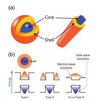
Fig. 2 (a) Schematic of core–shell nanoparticle and core–shell nanowire/nanorod. (b) Schematic representations of energy band diagrams and carrier localization in different types of core–shell structures.
