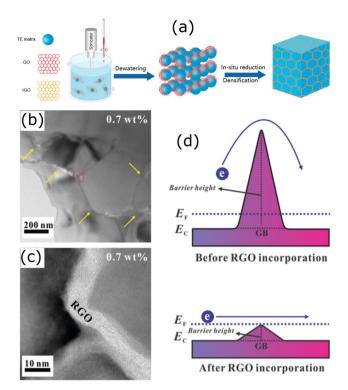
Fig. 16 (a) Schematic illustration of the synthesis of a bulk composite containing graphene (RGO) layer encapsulated grains (Reproduced with permission from ref. 183, Copyright 2020 American Chemical Society). (b and c) HRTEM micrographs of the STO-0.7 wt% RGO composite. (d) Schematic of double Schottky barrier of the STO-RGO composites. Reproduced with permission from ref. 171, Copyright 2019 Nature Publishing Group.
