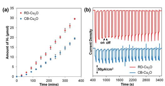
Fig. 2 (a) Time course of photocatalytic H<sub>2</sub> evolution during 6 hours of illumination and (b) PEC amperometric photocurrent densities of CB-Cu<sub>2</sub>O and RD-Cu<sub>2</sub>O.
