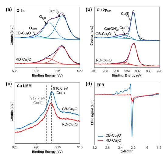
Fig. 5 (a) O1s, (b) Cu2p<sub>3/2</sub>, (c) Cu LMM spectra from XPS measurement and (d) EPR spectra for CB-Cu<sub>2</sub>O and RD-Cu<sub>2</sub>O.
