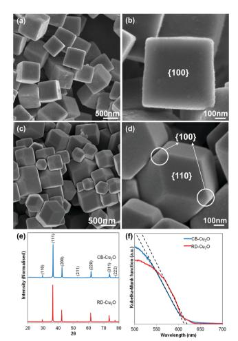
Fig. 1 SEM images of (a and b) cubic  $Cu_2O$  with dominant {100} facet, (c and d) rhombic dodecahedral  $Cu_2O$  with dominant {110} facet, (e) XRD patterns and (f) UV-Vis absorption spectra of CB- $Cu_2O$  and RD- $Cu_2O$  converted using Kubelka–Munk transformation.
