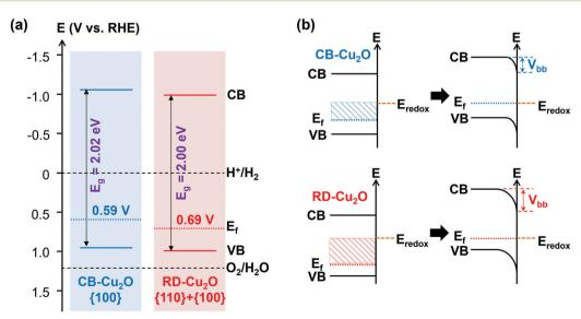
Fig. 4 (a) Postulated electronic band structures and (b) expected downward band bending at the semiconductor/electrolyte junctions of CB- $Cu_2O$  and RD- $Cu_2O$ .
