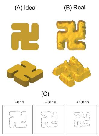
Fig. 2 A plan and 3-D view of the (A) ideal and (B) real models of LH gammadion nanostructures used in numerical simulations. (C) Cut slice profile of the 'real' structure 0, 50 and 100 nm above the glass substrate. The structure shows significant sloping.
