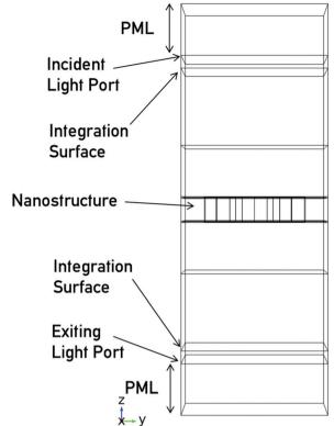
Fig. 8 Geometry of the simulation with PML, light ports and integration surfaces identified
