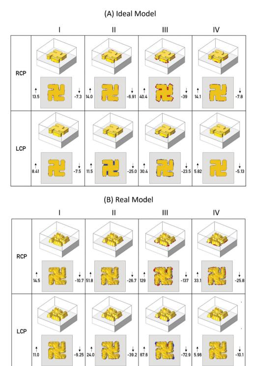
Fig. 6 Time averaged normalised (with RCP) optical chirality plots above a threshold of 2.5 (red) (-2.5 (blue)) for (A) real and (B) ideal models. The minimum (1) and maximum (1) values for each resonance and light handedness are included.
