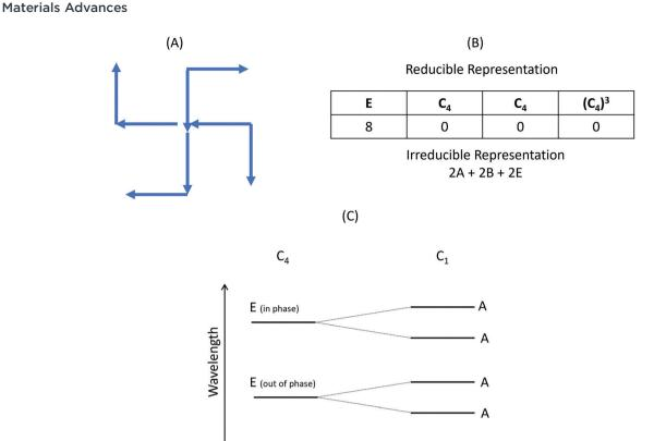
Fig. 7 (A) Basis set of vectors used in the symmetry analysis; (B) the reducible and irreducible representations produced by the basis set of vectors. (C) An energy level diagram showing the effects of a symmetry reducing perturbation.
