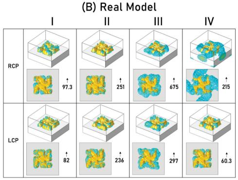
Fig. 4 3-D electric field plots for incident LCP and RCP light, with a 10 V m<sup>-1</sup> threshold, generated from (A) real (B) idealised models. The largest value of |E| is given with an up arrow in each inset.
