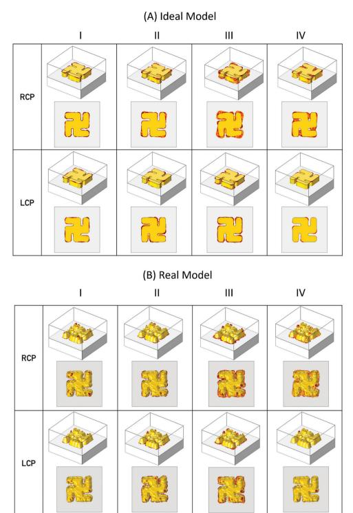
Fig. 5 3-D electric field plots for incident LCP and RCP light, with a 20 V m<sup>-1</sup> threshold, generated from (A) real (B) idealised models.
