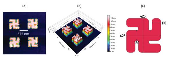
Fig. 1 AFM images of a LH gammadion displayed in (A) plane and (B) 3-D topological views; (C) is a schematic of the structures which displays relevant dimensions
