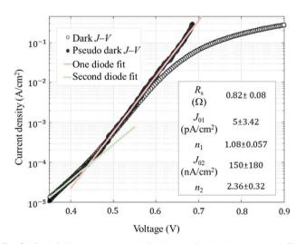
Fig. 6 Dark J-V and pseudo dark J-V curves for the best solar cell. The pseudo J-V characteristic, free of series resistance effects, is determined from Suns- $V_{\rm oc}$  measurements. The fitting parameters are shown in the inset.
