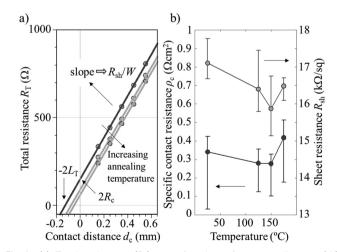
(a) Total resistance ( $R_T$ ) as a function of contact distance ( $d_c$ ) obtained from corresponding I-V curves for the ALD V2O5 film contacted with ITO/Ag. (b) Specific contact resistivity ( $\rho_c$ ) and Sheet resistance ( $R_{sh}$ ) dependence on annealing temperature extracted from TLM measurements.
