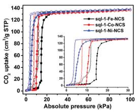
Fig. 2  $CO_2$  sorption isotherms for **sql-1-M-NCS** (M = Fe, Co, and Ni) at 195 K. The solid and open symbols represent adsorption and desorption branches, respectively.
