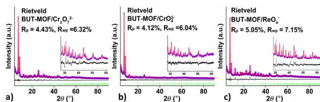
Fig. 9 Rietveld plots of (a) **BUT-MOF/Cr<sub>2</sub>O<sub>7</sub><sup>2-</sup>**, (b) **BUT-MOF/CrO<sub>4</sub><sup>2-</sup>** and (c) **BUT-MOF/ReO<sub>4</sub><sup>-</sup>**. Blue crosses: experimental points; red line: calculated pattern; violet line: difference pattern (exp. – calc.); green bars: Bragg positions. Inset: Magnification of the  $2\theta$  region  $30\text{--}60^\circ$ .
