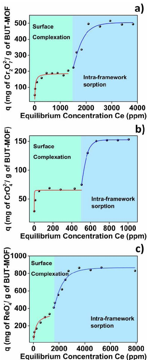
Fig. 3 (a)  $\text{Cr}_2\text{O}_7^{2-}$ , (b)  $\text{CrO}_4^{2-}$  and (c)  $\text{ReO}_4^-$  isotherm sorption data for **BUT-MOF** fitting with the various models. Red: Langmuir model; blue: Langmuir-Freundlich model.
