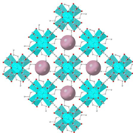
**Fig. 1** Representation of the framework structure of **BUT-MOF** (C, gray; O, red; N, blue; and Zr turquoise). The H atoms and the solvent molecules in the structural representation of **BUT-MOF** were omitted for clarity. The large plum balls indicate the pores in the structure of **BUT-MOF**.
