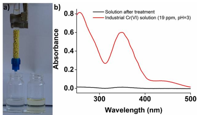
Fig. 7 (a) Cr(VI) industrial waste sorption by the column filled with **BUT-MOF**/calcium alginate beads (initial Cr(VI) concentration = 19 ppm, pH = 3, 480 mg of sorbent) and (b) UV-Vis spectra of the Cr(VI) industrial waste solution before and after treatment.
