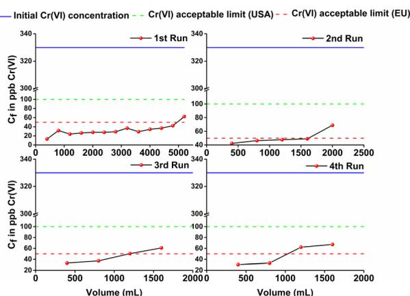
Fig. 8 Column sorption data with chrome-plating wastewater sample (flow rate 2.5 mL min<sup>-1</sup>) containing 330 ppb of Cr(VI).  $V_{\text{eff}}$  and  $C_{\text{eff}}$  are the volume (mL) and Cr(VI) concentration (ppb) of the solution passed through the column (*i.e.* effluent), respectively.
