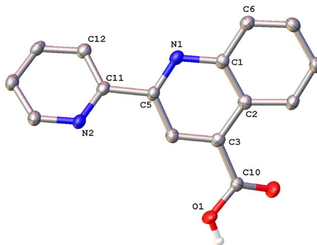
**Fig. 1** Molecular structure of **pqca**; ellipsoids are plotted at the 50% probability level. H atoms except those in the COOH groups are omitted. Selected bond lengths (Å) and angles (°): O(1)–C(10) 1.317(3); O(2)–C(10) 1.214(3); N(1)–C(5) 1.311(4); N(2)–C(11) 1.337(4); C(5)–C(11) 1.503(4); C(5)–N(1)–C(1) 117.9(2); C(11)–N(2)–C(15) 118.5(2); O(2)–C(10)–O(1) 124.1(3).
