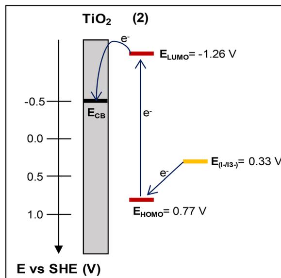
**Fig. 12** The energy diagram of the photoelectrode electrolyte interface depicting the HOMO–LUMO energy levels of dye (2) *vs.* the conduction band (CB) level of TiO<sub>2</sub> and the redox potential of  $I^-/I_3^-$ .
