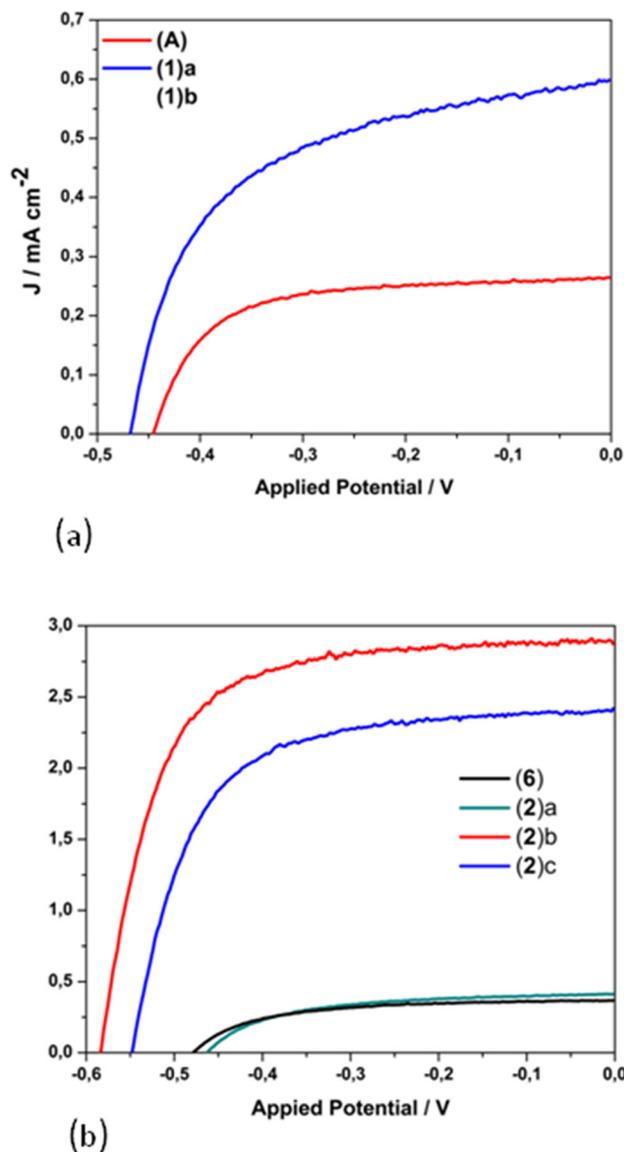
Fig. 13  $J$ – $V$  curves for the copper(I)-based dyes 1, [Cu(pqcame<sub>2</sub>)]PF<sub>6</sub> (A) (a); 2 and 6 (b). Lower case letters highlight the different architecture of the semiconductor material of the anode, dyed with 1 and 2, as reported in Table 2.
