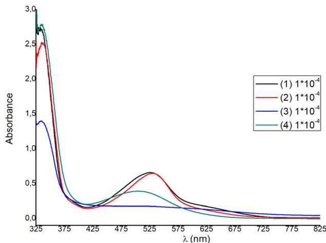
Fig. 9 Absorption spectra of compounds 1–4 in Me<sub>2</sub>CO at 298 K.
