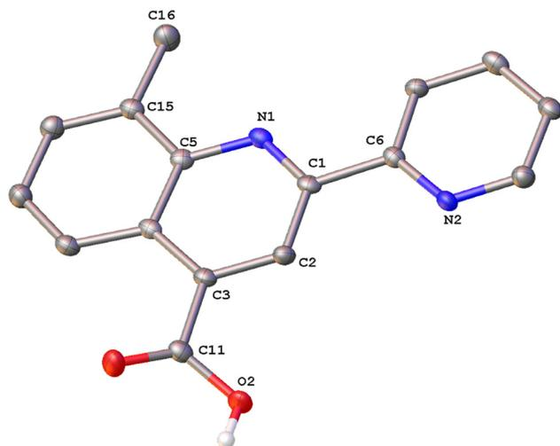
**Fig. 3** Molecular structure of 8-Mepqca; ellipsoids are plotted at the 50% probability level. H atoms, except those in the COOH groups are omitted.
