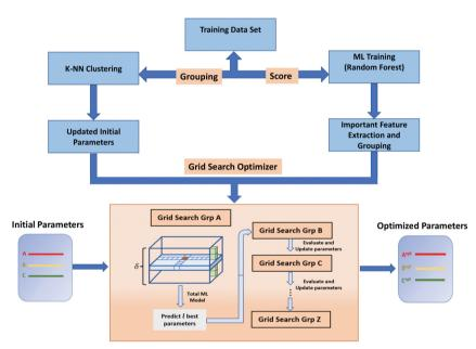
Fig. 37 Illustration showing entire the machine learning scheme. Figure adapted from ref. 576
