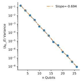
Fig. 43 The plot shows sample variance of the gradient of a two-local Pauli term plotted as a function of the number of gubits on a semi-log plot. Reprinted from ref. 728 with permission under Creative Commons Attribution 4.0 International License
