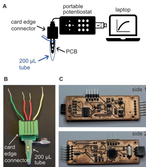
**Fig. 2** Schematics and pictures of the electroanalytical device. (A) Schematics of the potentiostat showing connection with the computer and the PCB for sample analysis. (B) Picture of the PCB with a card edge connector, fitting inside a 200  $\mu\text{L}$  tube. The size of a PCB is  $1.2 \times 3.1$  cm. (C) Picture of the main components of the potentiostat. The size of the potentiostat is  $2.3 \times 7$  cm.
