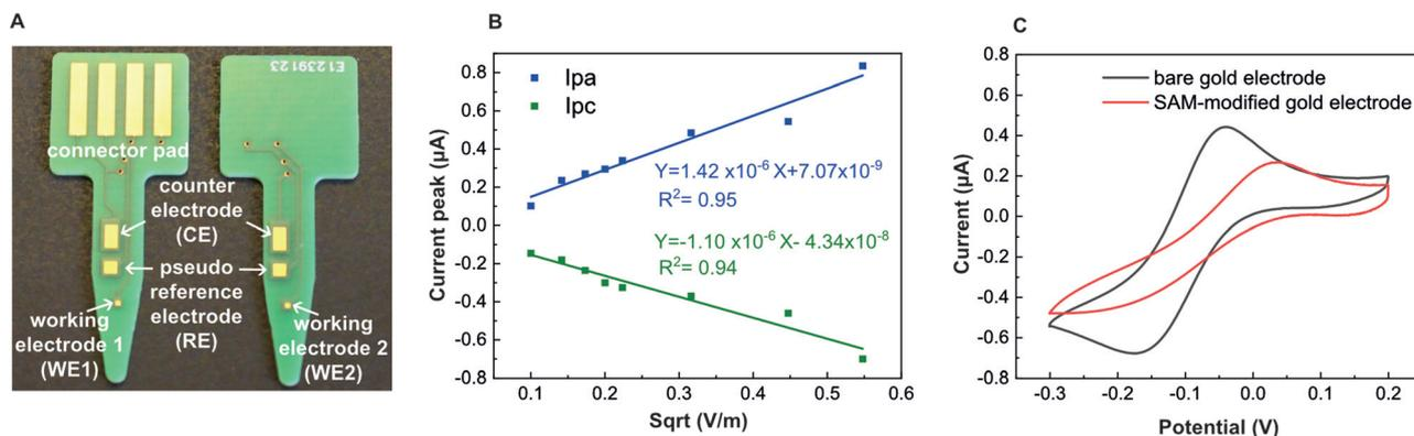
**Fig. 1** Design and electrochemical characterization of the PCBs. (A) Each PCB has 4 gold electrodes. (B) Randles–Sevcik plots of bare gold electrodes and SAM-modified gold electrodes after conducting CVs in 5 mM ferricyanide at different scan rates ( $10 \text{ mV s}^{-1}$ – $300 \text{ mV s}^{-1}$ ) ( $n = 3$ ). (C) Representative CV in 5 mM ferricyanide (scan rate of  $30 \text{ mV s}^{-1}$ ) after gold electroplating: bare gold electrode and SAM-modified gold electrode.
