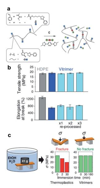
Fig. 7 (a) Synthetic scheme for various copolymers containing pendant dioxaborolanes (PS, PMMA, and HDPE). (b) Tensile properties of HDPE (gray column) and HDPE vitrimers (pristine: blue, reprocessed: light blue). (c) Environmental stress-cracking resistance of PS vitrimer. Reproduced from ref. 50 with permission from the AAAS.
