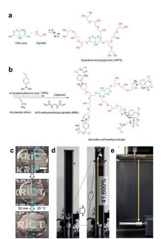
Fig. 13 (a) Synthesis of LMPG using cationic ring-opening polymerization. (b) Preparation of a hydrogel using the radical polymerization of VBA and acrylamide. (c) Photographs of the self-healing process of the hydrogel, which self-heals after 30 min at room temperature. (d) Photographs before and after stretching the hydrogel  $\sim\!416$  times its initial length using a UTM. (e) A photograph of the hydrogel spinning process. Reproduced from ref. 82 with permission from the Springer Nature.
