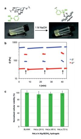
Fig. 15 (a) Gelation of an agueous solution of alginate modified with boronic acid upon increasing the pH. (b) Oscillatory rheological tests showing the thixotropy of the hydrogel. The arrows indicate the increase in the shear strain to 500%. (c) In vitro cytotoxicity of the hydrogel cultured with HeLa cells after 24, 48, and 72 h of incubation. Reproduced from ref. 93 with permission from the RSC.
