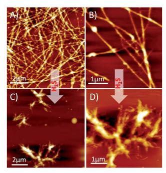
Fig. 2 AFM images of HSNPc and HSNPc with H<sub>2</sub>S. (A) AFM image shows a fibrous network of HSNPc and (B) its magnified image shows straight fibers. (C) and (D) Shows the change in self-assembly after H<sub>2</sub>S treatment.
