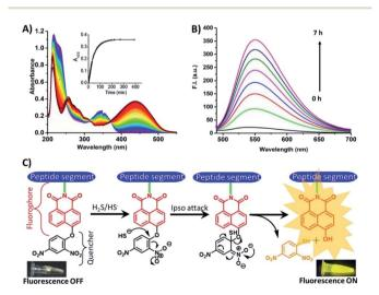
Fig. 1 Time-dependent UV-Vis and fluorescence spectra of HSNPc, showing sensitivity in the presence of H<sub>2</sub>S. (A) UV-Vis, (B) fluorescence and (C) fluorescence ON and OFF mechanisms.
