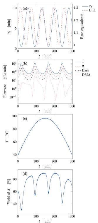
Fig. 5 Time variation of the input and output parameters for run 3 of Table 1: (a) instantaneous residence time and base equivalents; (b) species flowrate; (c) measured temperature; (d) measured yield of the desired product.
