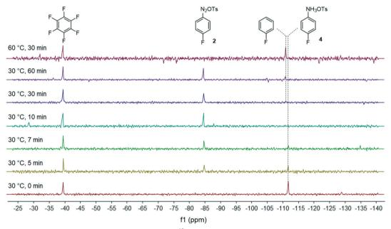
Fig. 3 Monitoring of the diazonium salt formation in THF by in-line <sup>19</sup>F NMR analysis at 40.88 MHz.
