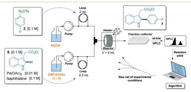
Scheme 2 Reaction setup for the optimization of indole 6.
