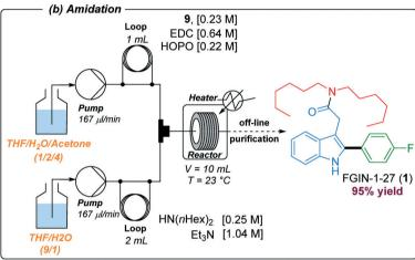
Scheme 3 Reaction setups used for preparing acid 9 and FGIN-1-27 (1).
