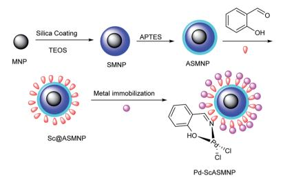
Scheme 19 The preparation of Pd-Sc@ASMNPs nanocatalyst.
