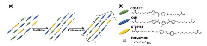
Fig. 1 (a) Generalized synthetic approach to prepare azobenzene-functionalized liquid crystalline elastomers (azo-LCE) by a one-pot, two-step polymerization method utilizing aza-Michael addition and subsequent photopolymerization. (b) The liquid crystalline monomers C6BAPE, C6M, and ST04181 were mixed with hexylamine to prepare monodomain azobenzene-functionalized LCE.
