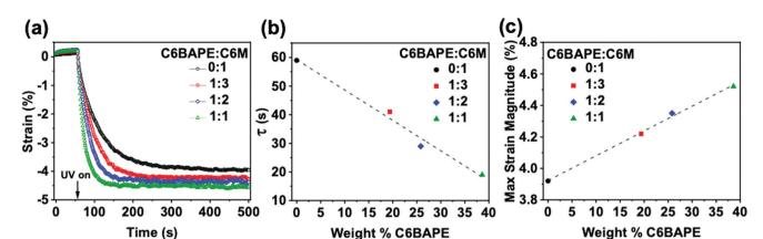
Fig. 4 (a) Photomechanical strain generated by azobenzene-functionalized LCE. (0.001 N constant force, 50 mW cm<sup>-2</sup>, 365 nm light exposure at 60 s) (b) Time constants as a function of C6BAPE concentration calculated from exponential fitting of photomechanical strain curve. (c) Maximum photomechanical strain as a function of C6BAPE concentration.
