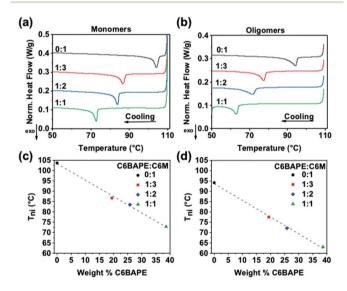
Fig. 2 DSC thermograms of (a) monomer mixtures and (b) oligomers used to prepare monodomain azobenzene-functionalized LCE. The  $T_{\rm ni}$ of these materials is plotted as a function of C6BAPE concentration for (c) monomer mixtures and (d) oligomers.
