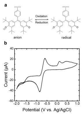
**Fig. 4** (a) The reversible redox reaction of PGMS. (b) Cyclic voltammogram of PGMS-39 (radical content 29%) on a gold working electrode using platinum as the counter electrode, recorded at a scan rate of 0.1 V s<sup>-1</sup> in 0.1 M tetrabutylammonium hexafluorophosphate (TBAPF<sub>6</sub>) in N,N-dimethylformamide (DMF). The voltammogram shown was obtained after 5 conditioning cycles.
