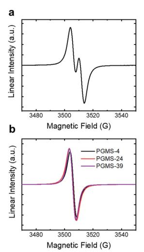
**Fig. 3** The normalized EPR spectra of (a) the small molecule galvinoxyl radical in toluene and (b) PGMS-4, PGMS-24, and PGMS-39 radical polymers in toluene
