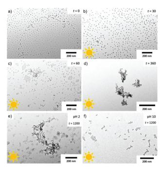
Fig. 5 pH-Dependent irradiation of P1 micelles ( $c = 0.1 \text{ mg mL}^{-1}$ ) at pH 2 and pH 10. (a)-(e) TEM images of micelles/NPs with increasing irradiation time from 0 s to 1200 s. (f) PS NPs after irradiation for 1200 s.
