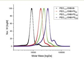
Fig. 2 GPC traces of PEO $_{113}$ -ONB-Br macroinitiator, PEO $_{113}$ -ONB-b-PS $_{90}$ , PEO $_{113}$ -ONB-b-PS $_{165}$ , and PEO $_{113}$ -ONB-b-PS $_{230}$ .
