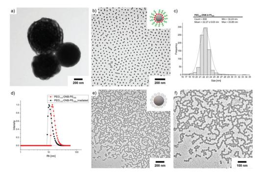
Fig. 4 Self-assembly and irradiation of PEO $_{113}$ -ONB-b-PS $_{165}$  (P2). (a) TEM of P2 after dialysis from THF into water. (b) TEM of P2 after dialysis from THF into acetone/IPA (80/20 v/v) and then into water. (c) Core size distribution of P2 averaged over 838 micelles. (d) DLS measurements of P2 before (red) and after irradiation (black) with UV light (365 nm) for 20 min. (e and f) TEM of PS NPs after irradiation.
