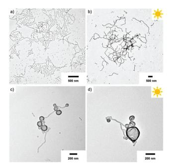
Fig. 6 Morphologies of PEO<sub>113</sub>-ONB-b PS<sub>x</sub> BCPs in water. TEM of P2 cylinder micelles at  $c = 0.1 \text{ mg mL}^{-1}$  before irradiation (a) and after irradiation (b). TEM of P3 vesicles at c = 0.1 mg mL<sup>-1</sup> before irradiation (c) and after irradiation (d).
