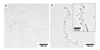
Fig. 7 TEM Characterization of PEO<sub>113</sub>-ONB-b-PS<sub>165</sub> (c = 0.1 mg mL<sup>-1</sup>, P2) mixed with AuNPs in a ratio of 1: 25.
