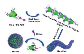
**Scheme 2** Preparation, self-assembly and disassembly processes of SKSPs.
