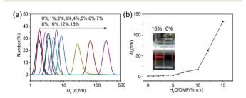
Fig. 1 Complexation and self-assembly of SKSPs. (a) DLS curves of CD-g-HPG-AZOs at various contents of H<sub>2</sub>O in DMF. (b) Dependence of  $D_h$  on the water content for CD-g-HPG-AZOs.
