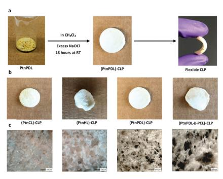
Fig. 3 (a) Image of PtnPDL-CLP flexible polymer. (b) Images of PtnCL, PtnHL, and P(tnPDL-b-CL) CLPs (c) Cross sectional morphology of cross-linked polymers under optical microscopy; magnification  $\times 10$ .
