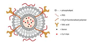
Fig. 13 Schematic representation of the boron-encapsulated liposome synthesised by Krishnan, Prasad and co-workers
