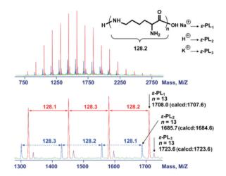
Fig. 6 MALDI-TOF-MS spectra of the chemosynthetic  $\varepsilon$ -PL. The sample was obtained by ROP followed by the removal of the protecting group. The red peaks correspond to  $\varepsilon$ -PL<sub>1</sub>. The blue peaks correspond to  $\varepsilon$ -PL<sub>2</sub>. The purple peaks correspond to ε-PL<sub>3</sub>. Reproduced from ref. 25 with permission from the Royal Society of Chemistry, copyright 2015.
