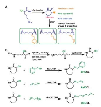
Scheme 3 (A) Lysine derivative cyclization and organocatalytic ringopening polymerization for the synthesis of functional polyamides. (B) Design and synthesis of functional cyclic lysine monomers. Reproduced from ref. 27 with permission from the American Chemical Society, copyright 2018.
