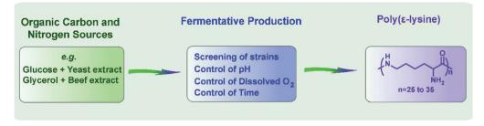
Fig. 2 Diagram for the biosynthesis of poly(ε-lysine) via fermentation.
