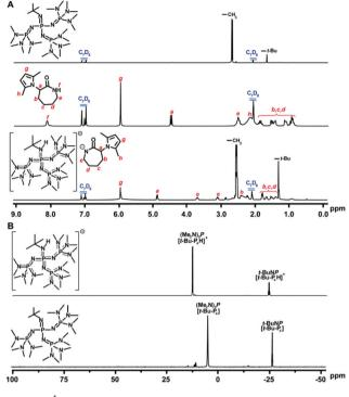
Fig. 4 (A)  $^{1}$ H NMR spectra (toluene- $d_{8}$ , 25  $^{\circ}$ C) of the reaction between t-BuP<sub>4</sub> and M5 (1:1). (B)  $^{31}$ P NMR spectra (toluene- $d_8$ , 25 °C) of the reaction between t-BuP4 and M5 (1:1). Reproduced from ref. 26 with permission from the American Chemical Society, copyright 2017.
