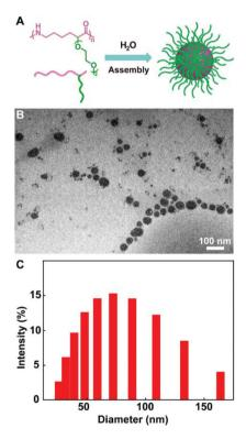
Fig. 8 Self-assembly of amphiphilic poly(OEGCL) into micelles. (A) Illustration on the formation of micelles. (B) TEM image of the micelle sample drop deposited from  $H_2O$  onto a carbon-coated copper grid; scale bar = 100 nm. (C) Size distribution of micelles measured by DLS. Reproduced from ref. 27 with permission from the American Chemical Society, copyright 2018.
