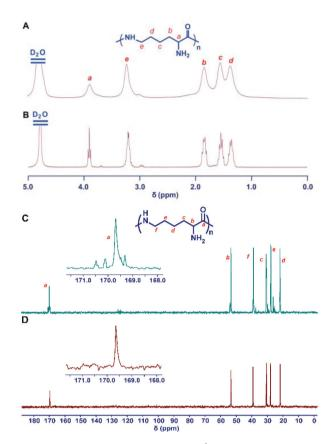
Fig. 5 Structure characterization of  $\epsilon$ -PL.  $^1$ H NMR spectra of chemosynthetic  $\epsilon\text{-PL}$  (A) and biosynthetic  $\epsilon\text{-PL}$  (B).  $^{13}\text{C}$  NMR spectra of chemosynthetic  $\varepsilon$ -PL (C) and biosynthetic  $\varepsilon$ -PL (D). All spectra were measured in D<sub>2</sub>O, pH 2 at room temperature. Reproduced from ref. 25 with permission from the Royal Society of Chemistry, copyright 2015.
