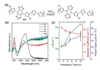
Fig. 13 (a) Structural representation of P5 before and after oxidative doping; (b) evolution of thin film UV-vis-NIR absorption spectra of P5 immersed in FeCl $_3$  solution as a function of time; (c) electrical conductivity, Seebeck coefficient, and power factor of P5 as a function of immersion doping time. Reproduced from ref. 94 with permission from the American Chemical Society.
