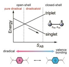
Fig. 2 Change of energies of triplet and singlet electron pairs with the increase in the one-electron overlap integral  $S_{\rm AB}$  and resonances between open-shell diradical and closed-shell quinoidal structures. Reproduced (adapted) from ref. 11 with permission from the Royal Society of Chemistry.
