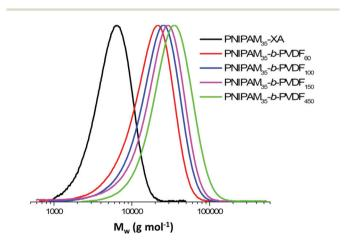
Fig. 1 Normalized SEC traces (viscometric detector) of: PNIPAM35-XA (black trace), PNIPAM<sub>35</sub>-b-PVDF<sub>60</sub> (red trace), PNIPAM<sub>35</sub>-b-PVDF<sub>100</sub> (blue trace), PNIPAM35-b-PVDF150 (pink trace) and PNIPAM35-b-PVDF450 (green trace) after purification by precipitation in chilled ether for PNIPAM or cold pentane for the BCPs.
