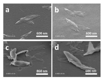
Fig. 7 SEM images of 2D lenticular objects prepared from: PNIPAM<sub>25</sub>b-PVDF<sub>35</sub> (a and b) and PNIPAM<sub>35</sub>-b-PVDF<sub>450</sub> (c and d).
