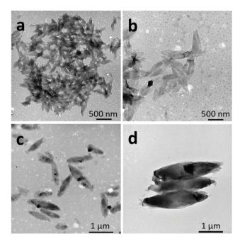
Fig. 6 TEM images of representative self-assembled 2D lenticular morphologies prepared from (a) PNIPAM35-b-PVDF60, (b) PNIPAM35-b- $PVDF_{100}$ , (c)  $PNIPAM_{35}$ -b- $PVDF_{150}$  and (d)  $PNIPAM_{35}$ -b- $PVDF_{450}$ . All samples were prepared via the solvent switch in acetone: water mixtures. Initial polymer concentration in acetone = 2 mg mL<sup>-1</sup>. Final concentration =  $0.4 \text{ mg mL}^{-1}$  in the acetone: water (1:4) mixture. Water addition rate =  $4 \text{ mL h}^{-1}$ .
