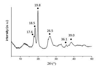
Fig. 8 X-Ray diffraction pattern of freeze-dried 2D lenticular aggregates obtained from PNIPAM<sub>35</sub>-b-PVDF<sub>100</sub> BCPs. The black dots indicate the characteristic peaks of the  $\alpha$ -phase of PVDF.
