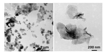
Fig. 4 TEM images of the bilayer aggregates obtained by the solvent switch of  $PNIPAM_{35}$ -b- $PVDF_{450}$ . Initial polymer concentration in THF = 2 mg mL $^{-1}$ . Final concentration = 0.4 mg mL $^{-1}$  in the THF: water (1:4) mixture. The water addition rate was 4 mL h<sup>-1</sup>.
