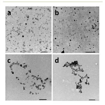
Fig. 2 TEM images of spherical aggregates prepared from (a) PNIPAM<sub>35</sub>-b-PVDF<sub>60</sub>, (b) PNIPAM<sub>35</sub>-b-PVDF<sub>100</sub>, (c) PNIPAM<sub>35</sub>-b-PVDF<sub>150</sub> and (d) PNIPAM<sub>35</sub>-b-PVDF<sub>450</sub>. All samples were prepared by nanoprecipitation in water from BCP solutions in DMF at 2 mg mL<sup>-1</sup> (final concentration = 0.1 mg mL<sup>-1</sup> in DMF: water (1:20)). Scale bars correspond to 200 nm.
