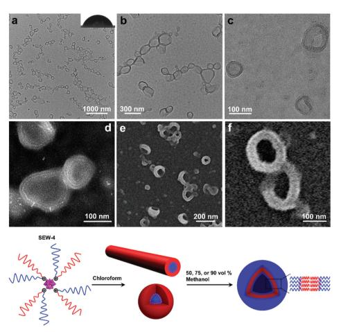
Fig. 5 BF-TEM (a–c), HAADF-STEM (d), and SEM images (e and f) show that SEW-4 self-assembled into regular bilayered vesicles with a PS<sub>57</sub> core and a  $[\alpha-SiW_{12}O_{40}]^{4-}$ /PEG<sub>45</sub> corona in the chloroform/methanol mixture solvent with a methanol content of 50 vol%. The inset (a) shows a water contact angle of 70°.
