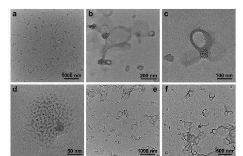
Fig. 6 Upon dispersing SEW-4 in the chloroform/methanol mixture solvent with a methanol volume of 10%, typical BF-TEM images show that regular bilayered vesicles coexisted with reverse solid spheres (a–d). When the methanol content was increased to 25 vol%, a pure phase of bilayered vesicles formed (e and f).
