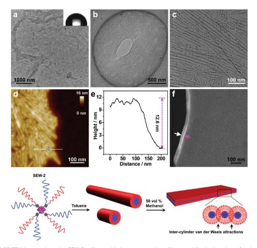
Fig. 3 (a, b, and c) BF-TEM images show that SEW-2 self-assembled to generate sheet-like assemblies in the toluene/methanol mixture solvent with a methanol percentage of 50 vol%. The inset (a) shows a water contact angle of 102°. A topographic AFM image (d) and its corresponding height profile (e) are shown for the sheet-like assemblies of SEW-2. (f) As indicated by the arrows in the SEM image, the cross-sectional area of the sheet was clearly captured.
