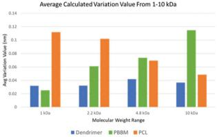
Fig. 4 Average  $R_h$  and size variation of each polymer across all tested molecular weight ranges using data from DOSY- $^1$ H NMR.
