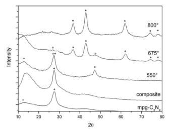
Fig. 6 Temperature-dependent powder XRD analysis of the TiO2 precursor/mpg-C<sub>3</sub>N<sub>4</sub> composites. (+) represents mpg-C<sub>3</sub>N<sub>4</sub>; (o), TiO<sub>2</sub>; and (\*), TiN. Reprinted from ref. 66 with permission from John Wiley and Sons, Copyright 2007.
