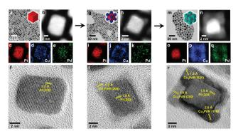
**Fig. 13** Time-dependent growth studies of  $Cu_3PdN$  on Pt nanocubes at 170 °C for (a-f) 5 min, (g-l) 10 min, and (m-r) 15 min. The data for each time point include (a, g, and m) TEM images, (b, h, and n) HAADF-STEM images, (c-e, i-k, and o-q) energy dispersive X-ray spectroscopy (STEM-EDS) element maps for Pt (red), Cu (blue), and Pd (green), and (f, l, and r) HRTEM images of individual particles. Reprinted with permission from ref. 119, Copyright 2019 American Chemical Society.
