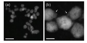
Fig. 3 High-angle annular dark-field scanning transmission electron microscopy (HAADF-STEM) images of the obtained TiN NCs via nonthermal plasma synthesis. Scale bars are (a) 20 nm and (b) 5 nm. Reprinted with permission from ref. 55. Copyright 2018 American Chemical Society.
