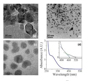
Fig. 8 TEM images of  $Ta_3N_5$  obtained by Ho et al. 87 (a) NPs obtained with TaCl<sub>5</sub> and (TMS)<sub>3</sub>N (scale 20 nm), (b) with Ta(NMe<sub>2</sub>)<sub>5</sub> and (TMS)<sub>3</sub>N (scale 20 nm) (c) with TaCl<sub>5</sub> and Li<sub>3</sub>N (scale 10 nm). (d) Absorption spectrum of the obtained 10 nm Ta<sub>3</sub>N<sub>5</sub>. The inset showing the two limiting regimes. Adapted with permission from ref. 87. Copyright 2010 American Chemical Society.
