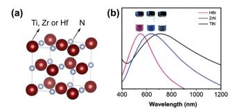
**Fig. 1** (a) Crystal structure of group 4 metal nitride. The metal is represented in purple and the nitrogen atom in grey. Structures plotted using VESTA. <sup>48</sup> Cif file obtained from ref. 49–51 (b) Absorption spectra of aqueous dispersions of TiN, ZrN, and HfN NCs. The inset shows a photograph of the NCs dispersed in water. Reprinted from ref. 40 with permission from John Wiley and Sons, Copyright 2019.
