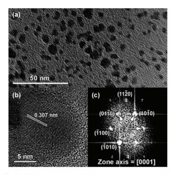
Fig. 21 TEM images of the colloidally stable InN obtained by Hsieh et al. after acid treatment. (a) Low magnification image, (b) high resolution image and (c) diffraction pattern obtained via fast Fourier transform (FFT). Reprinted with permission from ref. 173 with permission from the Royal Society of Chemistry.
