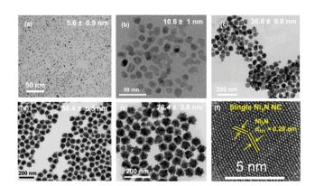
Fig. 10 TEM images of the different  $Ni_3N$  NCs obtained. (a) 5.6  $\pm$  0.9 nm, (b)  $10.6 \pm 1.0$  nm, (c)  $36.6 \pm 0.8$  nm, (d)  $56.4 \pm 6.5$  nm, and (e)  $76.4 \pm$ 3.8 nm. (f) High resolution transmission electron microscopy (HRTEM) image of a Ni<sub>3</sub>N nanocrystal with a size of 56.4 + 6.5 nm. Reprinted with permission from ref. 97. Copyright 2021 American Chemical Society.
