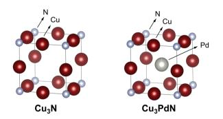
Fig. 11 Crystal structure of  $Cu_3N$  and the doped  $Cu_3PdN$ . The copper is represented in dark red, the palladium in grey and the nitrogen atom in cyan. Structures plotted using VESTA.<sup>48</sup> Cif file obtained from ref. 111 and 112.
