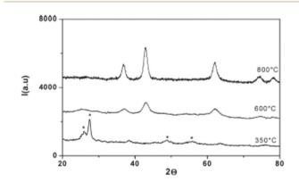
Fig. 7 XRD pattern of titanium-urea gels (R = 10) treated at different temperatures. The \* symbol refers to crystalline TiO2. Reprinted with permission from ref. 69. Copyright 2009 American Chemical Society.
