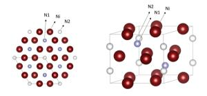
Fig. 9 Crystal structure of Ni<sub>3</sub>N. The nickel atoms are represented in dark red and the nitrogen atoms in cyan and white. Structures plotted using VESTA.48 Cif file obtained from ref. 89.
