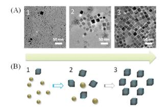
Fig. 14 (A) TEM of the  $\text{Cu}_3\text{N}$  NCs synthesized according to ref. 105, after 2, 5 and 10 min. (B) The proposed growth procedure of  $\text{Cu}_3\text{N}$  nanocubes. Reproduced from ref. 105 with permission from the Royal Society of Chemistry.
