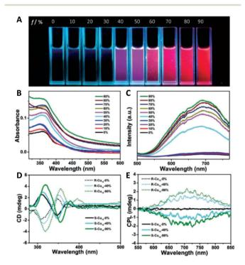
Fig. 24 (A) Photographs of fluorescent R-Cu $_{14}$  in solutions with different fractions of n-hexane. (B) UV/Vis absorption spectra, (C) emission spectra, (D) CD spectra, and (E) CPL spectra of R/S-Cu $_{14}$  in DCM/n-hexane mixtures with different (fv) values. Adapted with permission from ref. 173. Copyright 2019 Wiley-VCH Verlag GmbH & Co. KGaA, Weinheim
