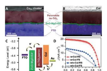
**Fig. 38** Device structure and cross-sectional SEM image of (A)  $\text{Cu}_{53}$  and (B) Cul on perovskite films. (C) Energy-level diagram of Cul-based perovskite solar cell (PSC). (D) Best J-V curves of devices with Cul (w-Cul) and without Cul (w/o-Cul). FS = forward scan, RS = reverse scan. Adapted with permission from ref. 194. Copyright 2019 Wiley-VCH Verlag GmbH &Co. KGaA, Weinheim.
