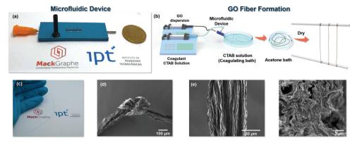
Fig. 1 (a) Photograph of the 3D hydrodynamic flow focusing microfluidic (3DHFFM) device fabricated to obtain the GO microfibers. (b) Illustration GO microfiber formation. (c) Photograph of the GO microfiber. SEM images of the GO microfibers (d) with an overhand knot, and (e) of the surface and (f) cross section. The GO microfibers are flexible, and their surfaces are not smooth, with many dentate-bends.
