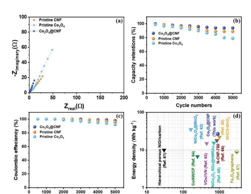
Fig. 7 Electrochemical performance of the SSC devices for the pristine  $Co_3O_4$  nanoparticles, pristine CNF and 1D  $Co_3O_4$ @CNF hybrid electrodes: (a) EIS plot, (b and c) capacity of retentions and coulombic efficiency of electrodes at 15 A g<sup>-1</sup> of current density over 5000 cycles and (d) Ragone plot.
