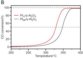
Fig. 22 (A) Schematic of the estimation of CO conversions over  $Pt_{17}/\gamma$ - $Al_2O_3$  or  $Pt_{NP}/\gamma$ - $Al_2O_3$  coated on a cordierite honeycomb substrate. (B) CO conversions over  $Pt_{17}/\gamma$ - $Al_2O_3$  or  $Pt_{NP}/\gamma$ - $Al_2O_3$ . Reproduced from ref. 235. Copyright 2020 Royal Society of Chemistry
