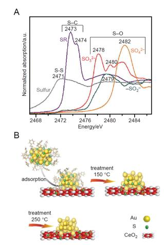
Fig. 10 (A) XANES spectra at S K-edge of different reference materials. (B) Schematic of thiolate ligands evolution upon NC deposition on CeO<sub>2</sub> and oxidative treatments. Reproduced from ref. 216. Copyright 2018 Wiley-VCH.
