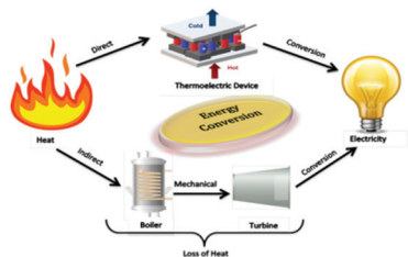
Fig. 1 Schematic representation of electricity generation by comparing the energy conversion between a thermoelectric device and conventional thermal plant.
