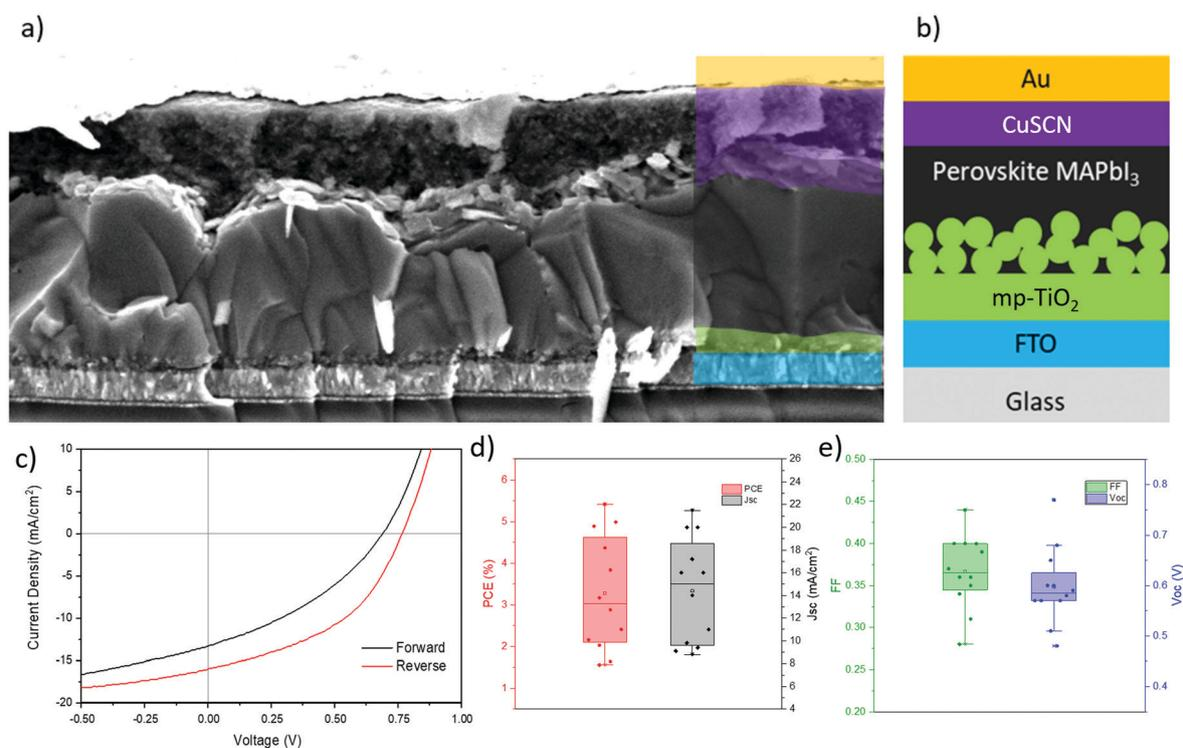
Fig. 2 (a) SEM of completed device cross-section. (b) Schematic of the device configuration used, corresponding to (a). (c)  $J-V$  Scan of champion cell showing forward and reverse scans. (d and e) Box-plots of PCE and  $J_{sc}$  (d) and FF and  $V_{oc}$  (e) of 12 cells, data taken from reverse scans.
