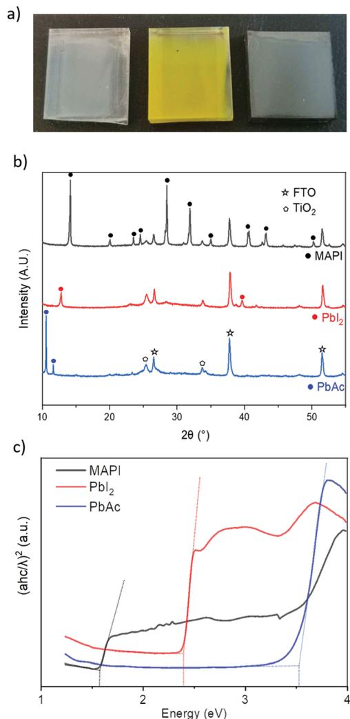
**Fig. 3** (a) Photographs of three films removed at different stages of the AACVD deposition (substrate size 12 mm × 12 mm). Left: Film after first step. Centre: Film halfway through MAI aerosol exposure. Right: Completed MAPI film (b) XRD patterns correspond to initial PbAc<sub>2</sub> film, PbI<sub>2</sub> intermediary and final MAPI film (c) Tauc plots of the three films calculated from absorption data.
