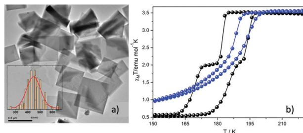
**Fig. 3** (a) TEM images of nanoplates of  $[\text{Fe}^{\text{II}}(2\text{-mpz})_2\text{Ni}(\text{CN})_4]$  and distribution of their sizes; (b) temperature dependence of the susceptibility data, in the form of  $\chi_M T$  for the nanoplates (blue spheres) and the bulk crystal (black spheres). Adapted from ref. 16 with permission from the American Chemical Society, copyright 2019.
