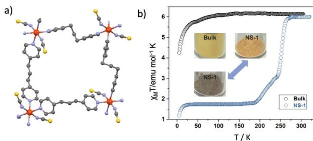
Fig. 7 (a) 2-D sheets are generated by the rhombic-grid unit of (4, 4)  $\text{Fe}(\text{1,3-bpp})_2$  color code: Fe, red; N, purple; S, yellow; C, grey; (b) temperature dependence of the susceptibility data, in the form of  $\chi_M T$ , of the exfoliated flakes (blue cycles) and the bulk crystals (black cycles) along with the temperature dependent color changes. Adapted from ref. 49 with permission from the American Chemical Society, copyright 2018.
