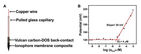
Fig. 5 Potentiometric characterization of the  $Cu^{2+}$  ISE: (A) schematic of the carbon-packed Cu(II) microsensor. (B) Potentiometric calibration of  $Cu^{2+}$  with the carbon-packed sensor. DOS: dioctyl sebacate. The sensors showed Nernstian slope of 29.3  $\pm$  2.9 mV/log [ $a_{Cu}^{2+}$ ] and detection limits of 3.5  $\pm$  1.0  $\mu$ M (number of experiments = 6).
