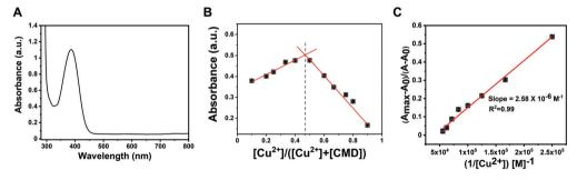
Fig. 2 UV-Vis characterization of metal-ligand binding: (A) UV-Vis spectra of the molecule ( $2 \times 10^{-5}$  M) with an absorption maximum centered at 387 nm. (B) Job's plot indicates that the ligand-to-metal binding ratio is 1:1 (number of experiments = 3). (C) The Benesi-Hildebrand plot provides a binding constant of the complexation ( $3.51 \times 10^5$  M<sup>-1</sup>) (number of experiments = 3).
