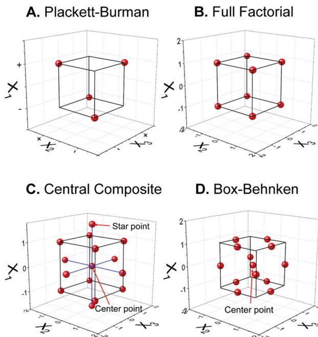
**Fig. 1** Two-level experimental designs illustrated for three parameters,  $X_1$ ,  $X_2$ , and  $X_3$ . (A) Plackett–Burman design, (B) full factorial design, (C) central composite design, and (D) Box–Behnken design.
