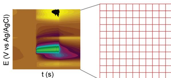
**Fig. 3** Classification of electrochemical data by their order. (A) Zero-order electrochemical data such as single pH measurement give a single data point. (B) First-order data such as those from DPV give a vector of current vs. potential. (C) Second-order data such as data from FSCV give a matrix of current vs. potential vs. time.
