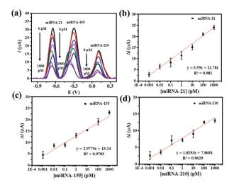
Fig. 5 (a) SWV responses of the proposed biosensor after incubation different concentrations of miRNA-21, miRNA-155, and miRNA-210, and (b), (c) and (d) corresponding calibration curves of the triplet assay towards miRNA-21, miRNA-155, and miRNA-210 respectively, in 10 mM PBS solution (pH 7.4).
