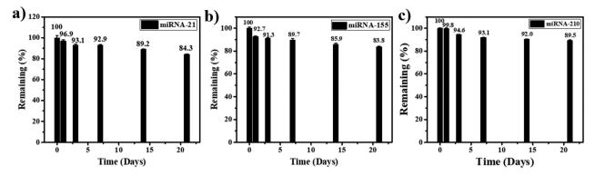
Fig. 7 Stability test of the proposed biosensor in the detection of (a) miRNA-21, (b) miRNA-155, and (c) miRNA-210 when the sensors are stored for 3 weeks.
